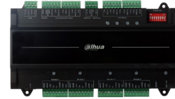
ASC2104B-T Slave Controller Four door one-way Users: 20,000 RS485/Wiegand(26/34) to readers; CAN bus;
