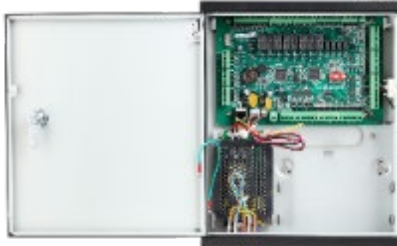
ASC2204C-H Master Controller Four door one-way Users: 200,000 RS485/Wiegand(26/34) to readers; TCP/IP to network; Onvif profile C, CGI;
