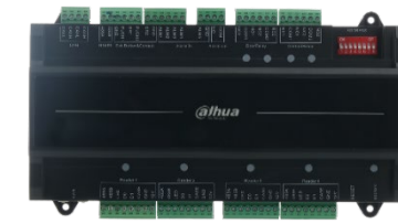
ASC2102B-T Slave Controller Two door two-way Users: 20,000 RS485/Wiegand(26/34) to readers; CAN bus;
